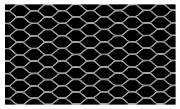
LW Pitch:25.40mmStrand Width:1.27mmSW Pitch:12.70mmThickness:1.20mmWeight:0.71 kg / m2Open Area:80%
